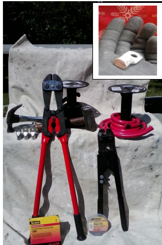
Tools of the trade: bolt cutters doubling as a cable cutter; heavy duty cable crimpers; 3lb sledge; claw hammer posing as a chasing hammer; 3/0 battery cables; 3/0 battery lugs w/ 1/4"; 5/16"; 3/8" eyelets. Inset: x-section of a crimped cable.
