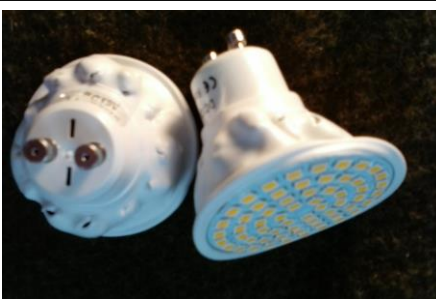
Melted 12Vdc bulbs from Banggood Tech.
